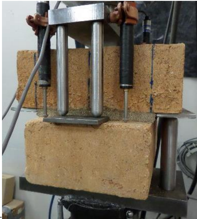
Figure 3.2 Couple specimen subject to uniaxial tensile loading: evaluation of bond strength at block/mortar interface.
