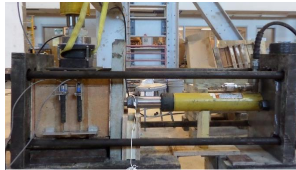
Figure 3.5 Triplet test specimens and setup.
