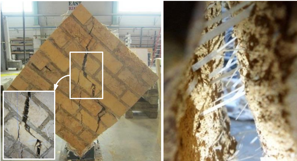
Figure 4.17 Representative failure mode for SREM specimens with close-up photograph of PET fibers bridging cracks.
