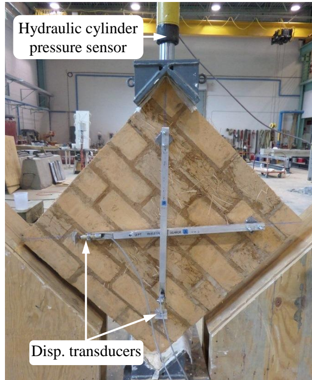
Figure 4.8 Diagonal compression test setup.
