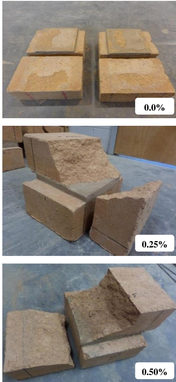
Figure 4.10 Representative failure mode for couplets with V_f = 0.0\% , 0.25% and 0.5%.
