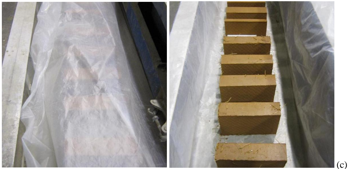
Figure 2.2 Manufacturing process: (a) Mechanical dry mixing and manual wet mixing, (b) casting and compression in hydraulic press, and (c) wet and dry curing.
