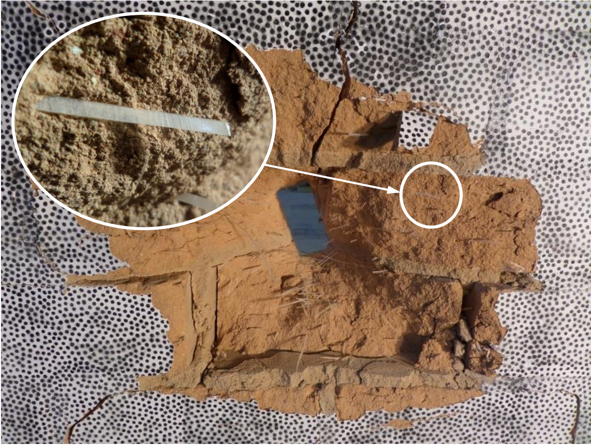
Figure 4.24 Photograph of post-impact damage showing broken PET fiber on SREM specimen.
