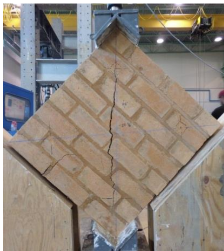
Figure 3.18 Diagonal compression test failure: (a) Specimen 1; (b) Specimen 2, with inset image showing cohesive bond failure, and (c) Specimen 3.
