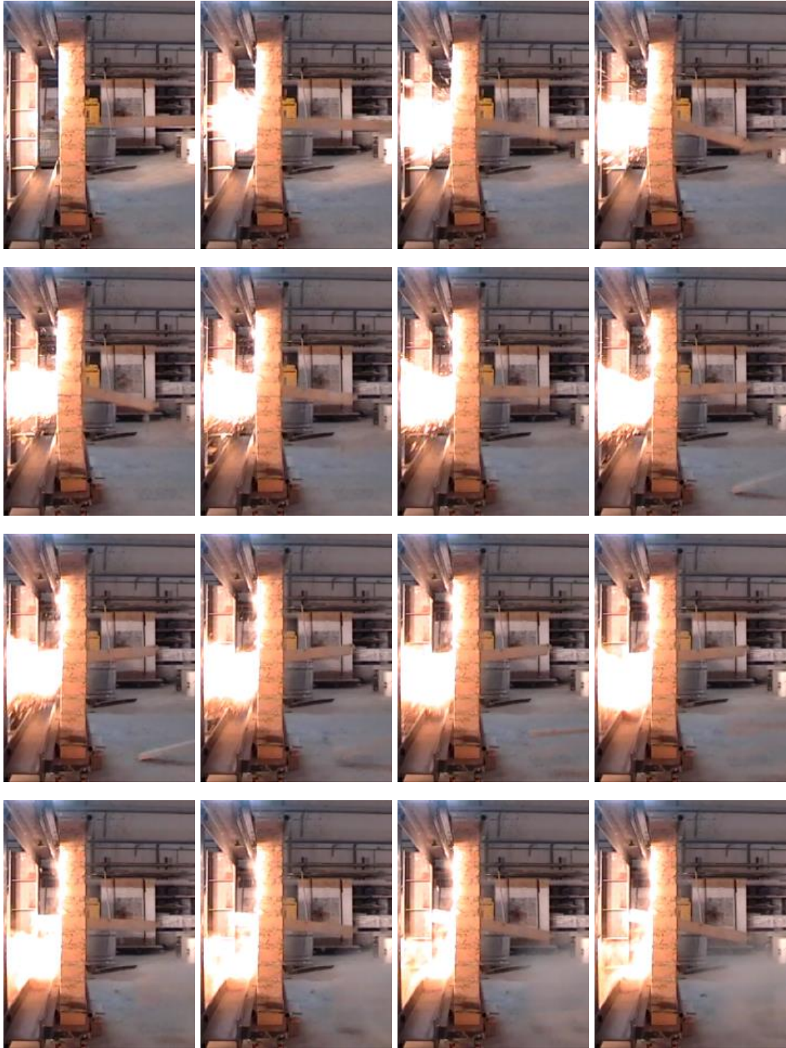
Figure 4.22 Impact sequence for SREM specimen showing missile stopped after partial penetration, (images every 33 ms).
