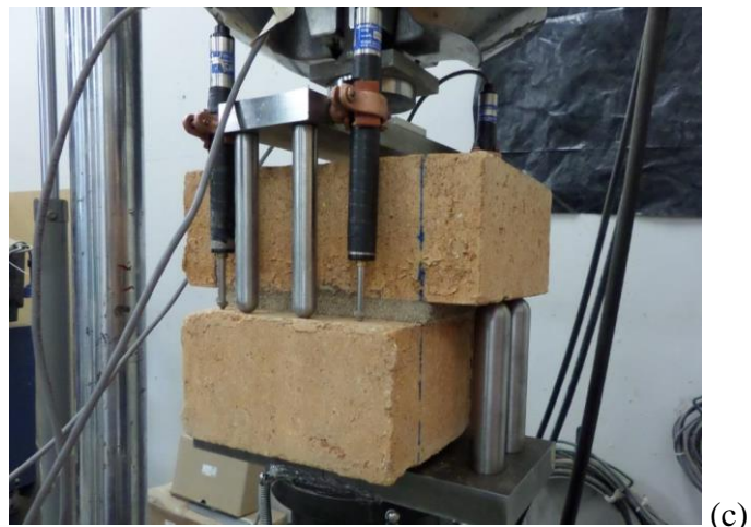
Figure 4.4 Mechanical characterization of fiber-reinforced mortar: (a) compression, (b) flexural, and (c) direct-tension (couplet) testing.
