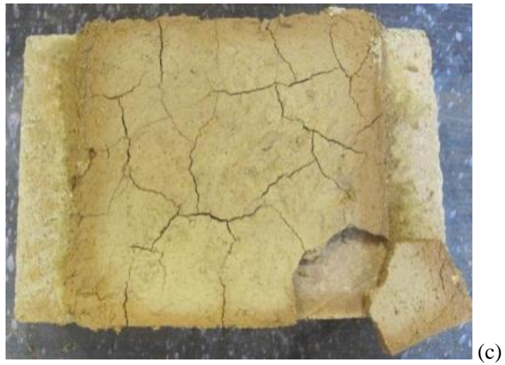
Figure 3.8 Shrinkage cracking at the block-mortar interface for SC10.
