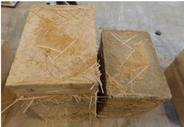
Figure 4.12 Representative failure mode for SREM specimens subject to out-of-plane loading.
